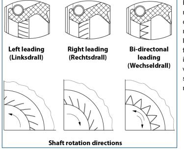
Radial shaft seals that are equipped with an oil return channel are called Left or Right leading type oil seals and also called as "drall" from Germanian naming. There are small notches on the back surface of the sealing lip, which pump the oil from the surface of the rotating shaft back to the inner side of the sealing edge during rotation. It is very important that this kind of special radial shaft seals is selected according to the direction of rotation of the shaft.
