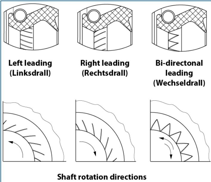
Radial shaft seals that are equipped with an oil return channel are called Left or Right leading type oil seals and also called as "drall" from Germanian naming. There are small notches on the back surface of the sealing lip, which pump the oil from the surface of the rotating shaft back to the inner side of the sealing edge during rotation. It is very important that this kind of special radial shaft seals is selected according to the direction of rotation of the shaft.
